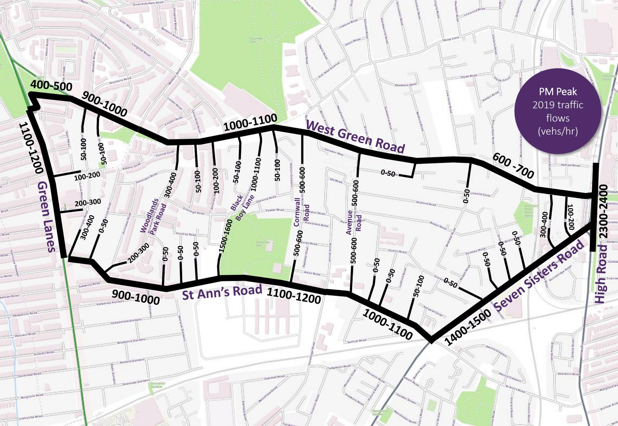
The plan below indicates the percentage changes in motor traffic flows, where all traffic reassigns onto the nearest available alternative route, which are the boundary roads on the edge of the LTN area. This assumes the boundary roads are able to accommodate this additional traffic.
