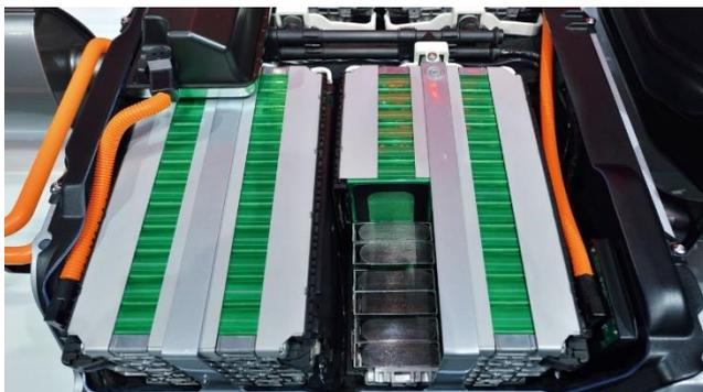
EV batteries are made up of a series of modules rather than being one large battery unit. This means that in the rare case of a cell in a module failing, the module in question can be replaced.
