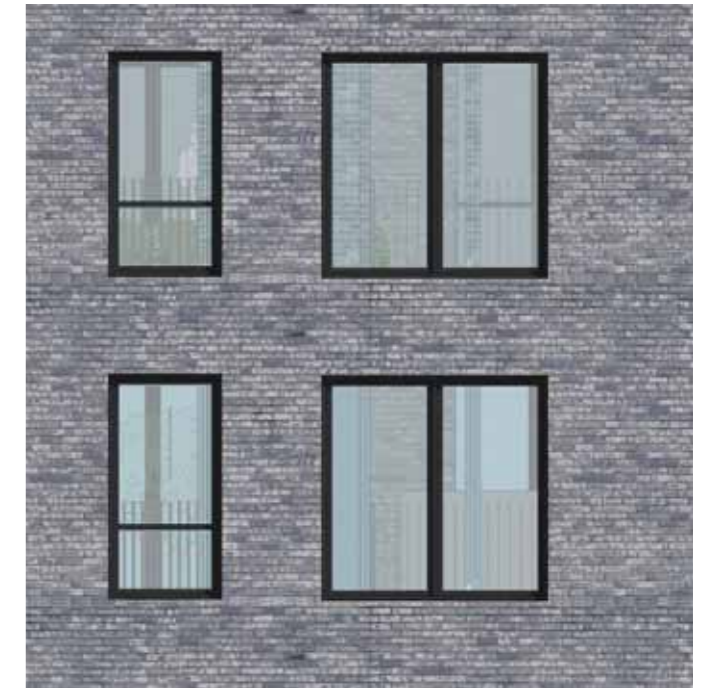
Variation 2: lighter tone grey brick with contrasting anthracite grey aluminium window frame
