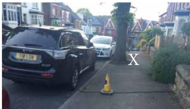
**Figure 2. What not to do: A bare cable trailing across the pavement is a safety hazard.**
