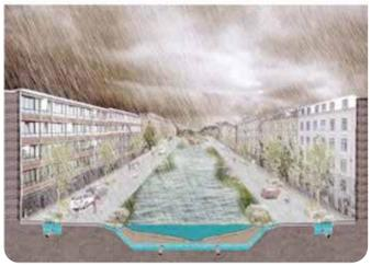
The system is being employed in a 45 hectare industrial estate in Malmo. The open storm water design successfully resulted in reduced peak-flows and reduced erosion risk for the Riseberga Creek. It now retains 90% of rainfall of a ten year peak event, whilst additionally providing recreational facilities to residents. The green facades showed they cooled the external surface of buildings by 8 °C, while the internal temperatures were reduced by between 1-1.5°C.
