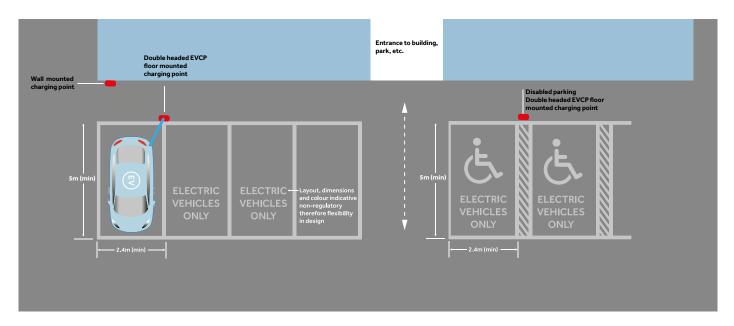
Figure 5. Car park layout for electric vehicle charging.
