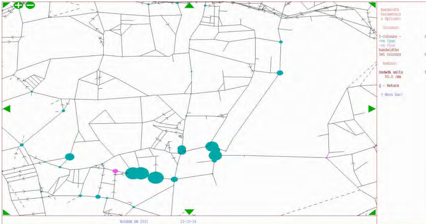
Figure 3.11: Change in junction delay (Do Something relative to Do Minimum scenario) – AM peak 9
