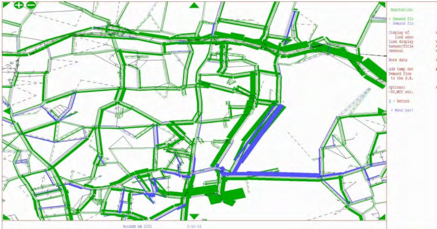
Figure 3.7: Change in total demand flow (Do Something relative to Do Minimum scenario) – AM peak 5
